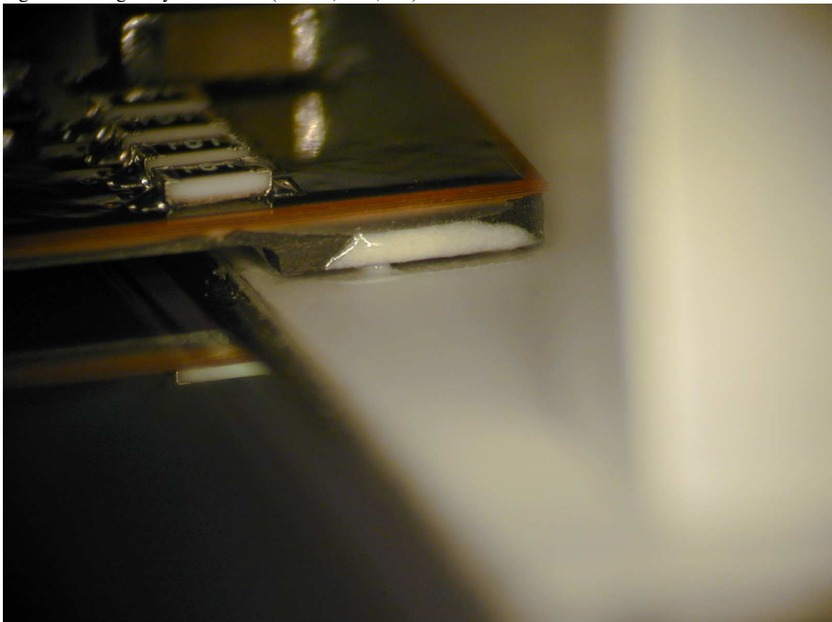
Fig.13. Gluing of hybrid foot b2 (bottom, near, right) of the module 20220170200043
