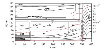
Figure 4: Yearly fluence of charged and neutral particles, translated into the 1-MeV neutrons, in the inner detector
