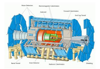
Figure 1: Overview of ATLAS detector at LHC
