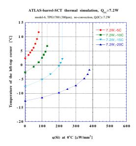
Figure 10: Thermal finite element analysis of the barrel module
