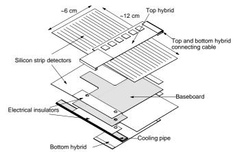
Figure 8: Construction of the barrel module
