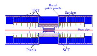
Figure 2: Layout of the inner detector
