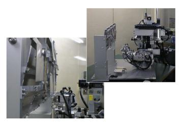
Figure 12: Module-mounting robot for the barrel cylindrical support structure. Top inset: overview together with a section of a dummy cylinder for development, and the bottom inset: the robot in action, holding a dummy module and moving toward the final position.
