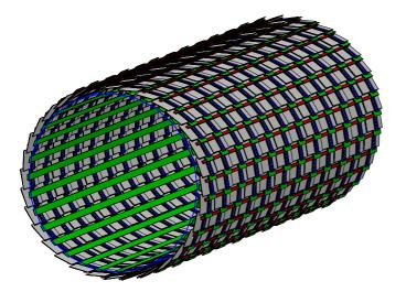
Figure 11: A graphical view of the barrel cylinder (B1). The carbon-fibre support cylinder is shown as a circle in an end.
