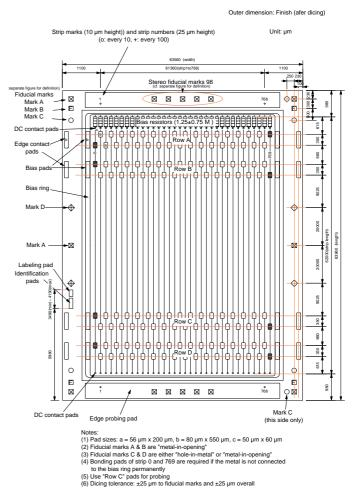
Figure 3: Layout of the Silicon microstrip sensor in the barrel section of the SCT
