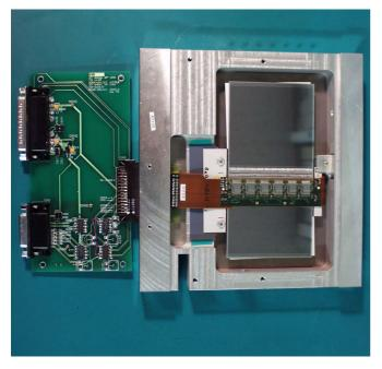
Figure 9: Fabricated barrel module being set in an Aluminium frame together with a communication card for testing
