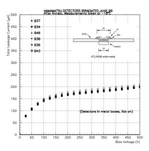
Figure 5: Leakage current vs bias voltage of the wide-metal design of the p-in-n sensor of the SCT, after  $3x10^{14}$  protons/cm<sup>2</sup> damage
