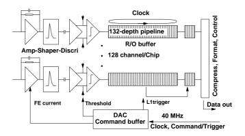
Figure 6: Schematic of the functionality of the front-end electronics
