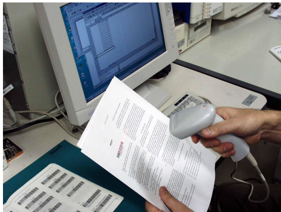
Figure 3: An example of the laser type barcode reader which scans the barcode and inputs to a spreadsheet
