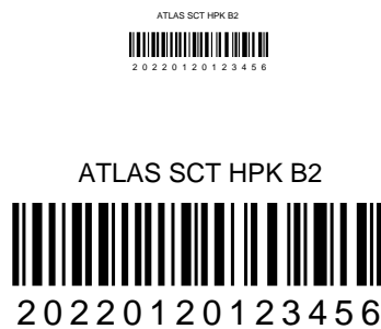
Figure 1: An example of the minimum size (top) and a typical size (bottom) of the SCT barcode
