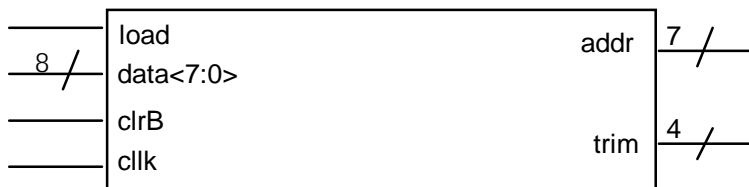
Figure 3.13A. Trim DAC Register Inputs/Outputs.
