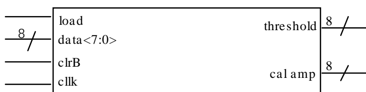
Figure 3.11. Threshold/Calibration DAC Register Inputs/Outputs.
