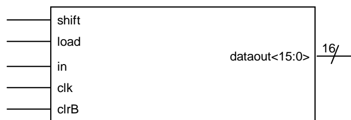
Figure 3.10. Configuration Register Inputs/Outputs.
