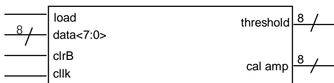
Figure 3.12. Threshold/Calibration DAC Register Inputs/Outputs.
