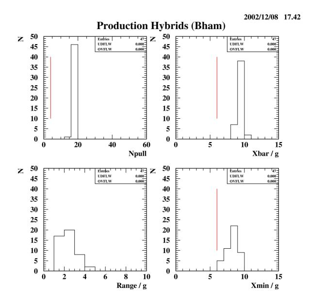
All pass X<sub>min</sub>>6g criteria We use at least 16 pull tests on each hybrid PA pull tests now being done systematically (not shown)
