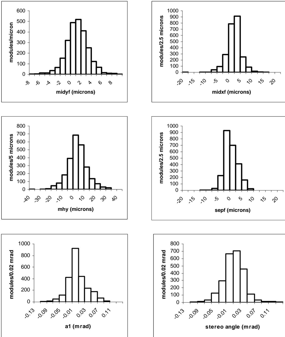
Fig. 19: The measured distributions of the deviations from their design values of a selection of module in-plane metrology parameters, whose definitions are shown in Fig. 16. Each plot is centred about the design value, with width  $\pm$  the specified tolerance (Table 12). The parameters are, from left to right: top row, *midyf*, *midxf*; middle row, *mhy*, *sepf*; bottom row, angles *a1* and half-stereo.
