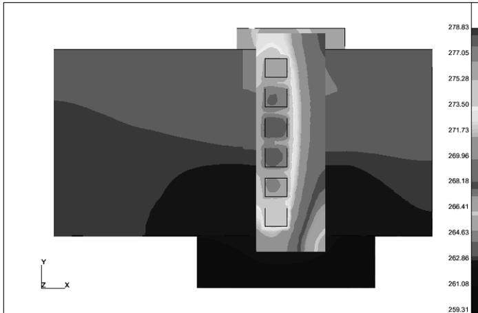
Fig. 12: An FEA simulation of the thermal profile of the SCT barrel module, with the maximum heat generation in the silicon microstrip sensors,  $120 \mu\text{W}/\text{mm}^2$ , a hybrid power consumption of 6 W, and a heat sink temperature of  $-14^\circ\text{C}$  at the cooling contact. The highest and the lowest temperatures are  $+5.7^\circ\text{C}$  and  $-13.8^\circ\text{C}$ , respectively.
