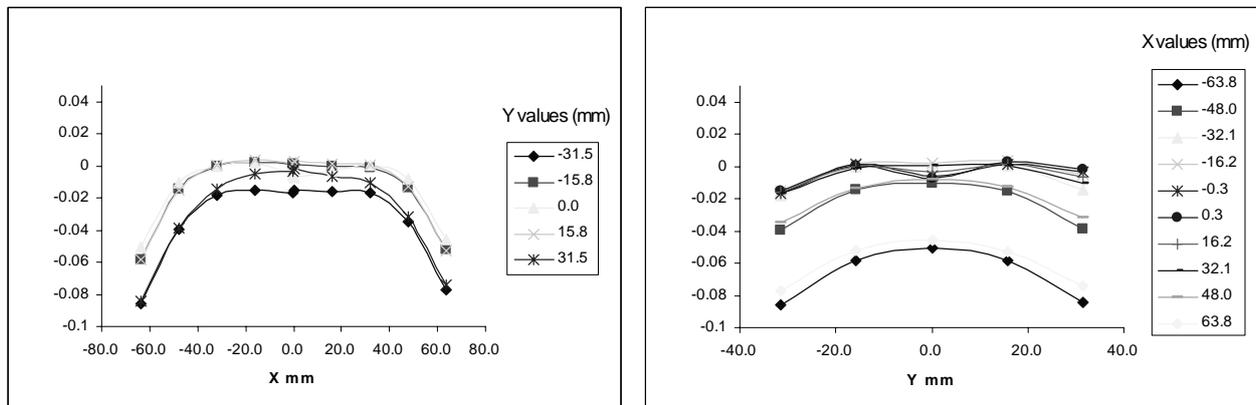
Fig. 17: The common  $Z$  profile (in mm) of the surface of the upper sensors for  $\langle 111 \rangle$  modules (see text). The lower surface is very similar, but with the opposite sign of  $Z$ . The left figure shows the profile along the length of the module ( $X$ ), at different transverse positions ( $Y$ ), and the right figure the profile across the module ( $Y$ ) at different longitudinal positions ( $X$ ).
