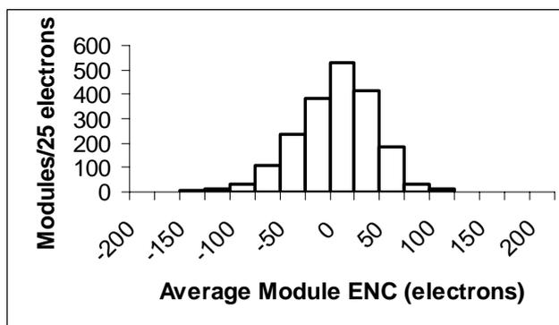
Fig. 30: The distribution of the difference in ENC, (barrel minus test box), measured at a hybrid thermistor temperature of  $\sim 28^\circ\text{C}$ , for all the modules mounted on the four SCT barrels.
