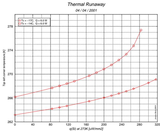
Fig. 13: Temperature of the hottest point in the sensors as a function of heat generation for a hybrid power of 6 W, with the heat sink temperatures of  $-14^\circ\text{C}$  (upper curve) and  $-17^\circ\text{C}$  (lower curve).
