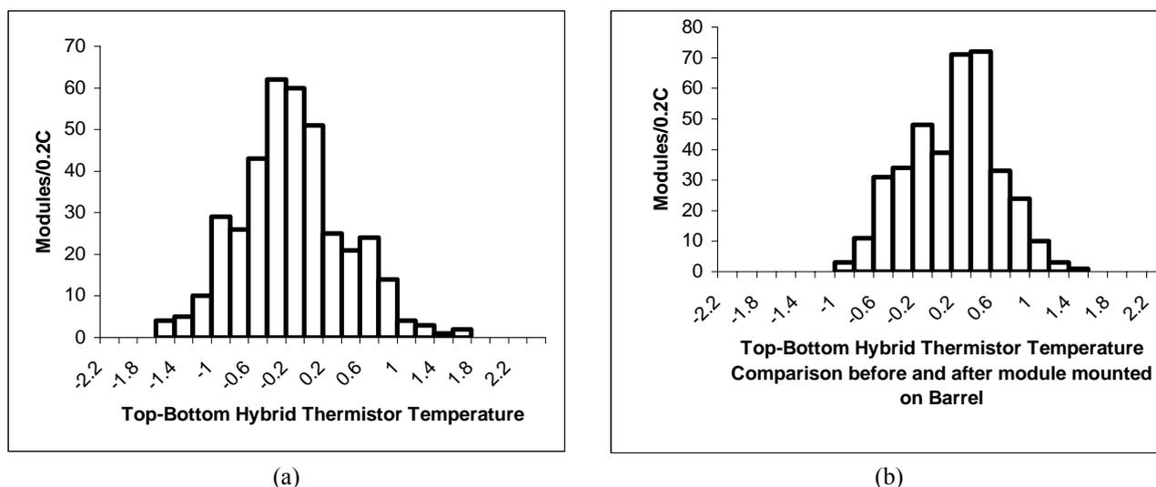
Fig. 29: (a) The difference in temperatures,  $dT$ , of the thermistors on the top and bottom faces of the module hybrid for modules operated before being mounted on Barrel 3 and (b) the change in recorded  $dT$  for these modules when being operated before and after mounting on Barrel 3.
