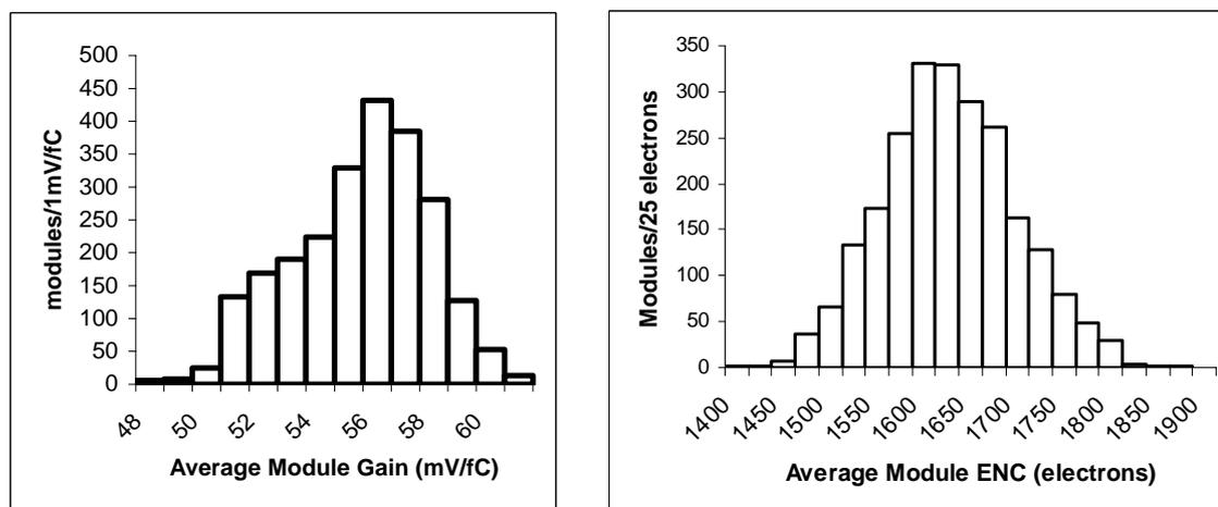
Fig. 25: Distributions of left: module gains, averaged over all channels in the module, and right: ENC, averaged over all channels in the module, at operational temperatures of  $\sim 28$ °C at the hybrid thermistors.
