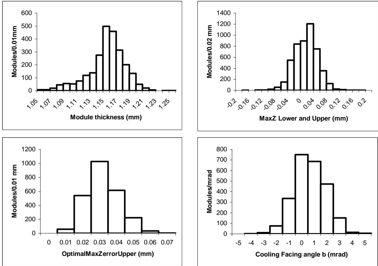
Fig. 20: The measured distributions of a selection of module Z (out-of-plane) metrology parameters, which are defined in Table 13. Each plot is centred about the design value, with width  $\pm$  the specified tolerance (Table 13). The parameters are, from left to right: top row, module thickness, maxZlower and maxZupper; bottom row, optimalMaxZerrorUpper, loCoolingFacing angle b.
