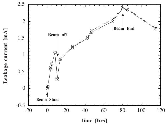
Fig. 2 Leakage current of a detector under irradiation. The bias voltage of ±40V is supplied during the irradiation (circle: n<sup>+</sup> back plane, cross: p<sup>+</sup> strip side). AC electrodes were grounded.
