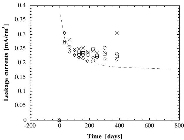
Fig. 6 Time variation of the leakage currents per unit volume for the four detectors at 0 °C. The dashed curve is the prediction of Fretwurst parameterization.
