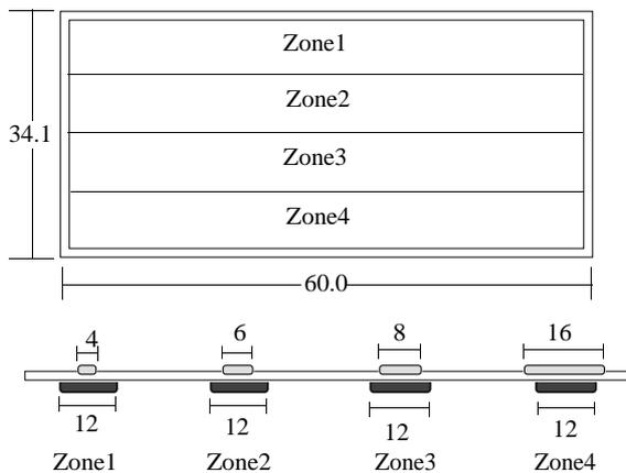
Fig. 1 Single-sided silicon microstrip detector under test. It has four zones of AC electrode widths (#1: 4μm, #2: 6μm, #3: 8μm, #4: 16μm) with a constant p-implant width of 12 μm. Four type of detectors were prepared with the AC coupling layers of SiO<sub>2</sub> or SiO<sub>2</sub>+Si<sub>3</sub>N<sub>4</sub>, and the passivation layer of SiO<sub>2</sub> or Si<sub>3</sub>N<sub>4</sub>.
