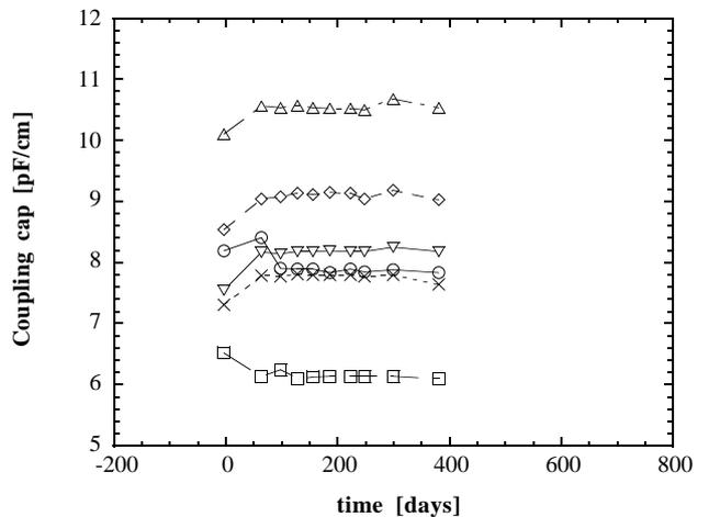
Fig. 8 Time variation of the AC coupling capacitances averaged per the zones and the insulators (O:  $\text{SiO}_2$ , ON:  $\text{SiO}_2+\text{Si}_3\text{N}_4$ ) (circle: 4 $\mu\text{m}$ -O, square: 4 $\mu\text{m}$ -ON, diamond: 6 $\mu\text{m}$ -O, cross: 8 $\mu\text{m}$ -ON, up-triangle: 16 $\mu\text{m}$ -O, down-triangle: 16 $\mu\text{m}$ -ON).
