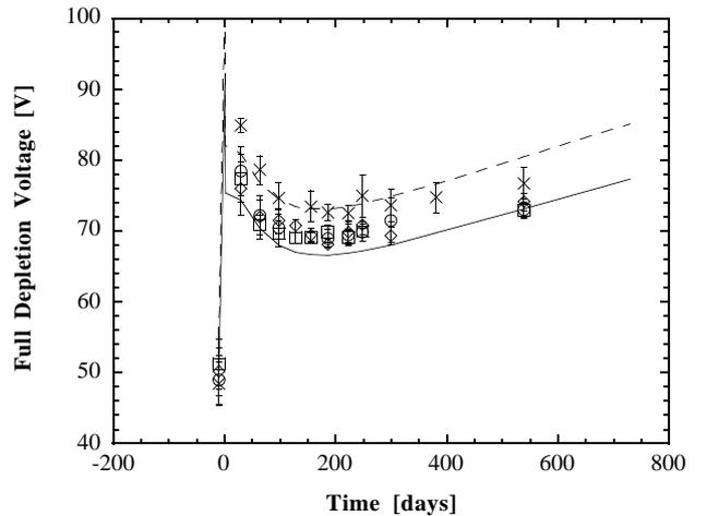
Fig. 4 Time variation of the full depletion voltage of the four detectors (cross: #1, diamond: #2, square: #3, circle: #4). Detectors were kept and measured at 0 °C after irradiation. The prediction of the Ziock's parameterization (solid curve) and a 10% increase for the strip detectors with a finite strip pitch and width (dashed).
