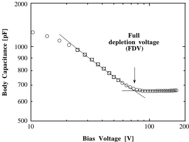
Fig. 3 Calculation of the full depletion voltage from the body capacitance measurement at the frequency of 10 kHz. The full depletion point is defined as the intersection point of the two fitted curves:  $y = a + b/\sqrt{x}$  to the under-depleted region,  $y = c$  to the over-depleted region. The data shown are for the detector #1, 185 days after irradiation.
