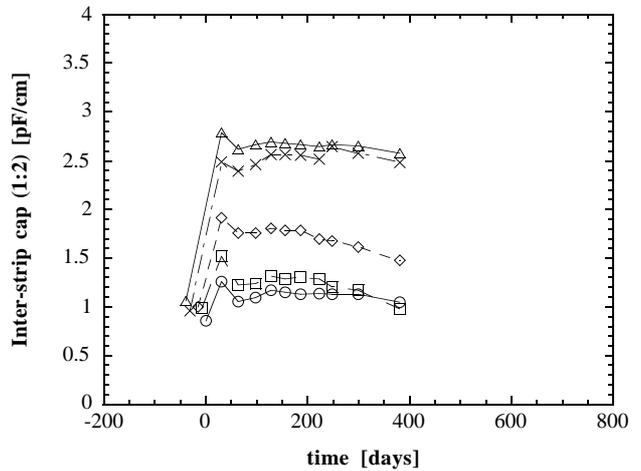
Fig. 7 Time variation of the inter-strip capacitances to the adjacent neighbors on both sides, averaged per zones (circle: 4 $\mu\text{m}$ , square: 6 $\mu\text{m}$ , diamond: 8 $\mu\text{m}$ , cross: 16 $\mu\text{m}$ - $\text{SiO}_2$  passivation, triangle: 16 $\mu\text{m}$ - $\text{Si}_3\text{N}_4$  passivation). The data before irradiation are displaced for readability.
