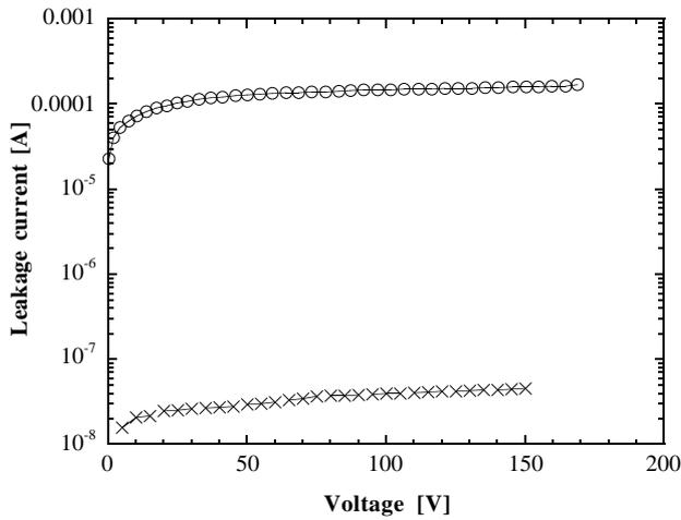
Fig. 5 Leakage current of a detector (#1) before irradiation (cross) and 185 days after irradiation (circle). Both currents were measured at 0 °C.
