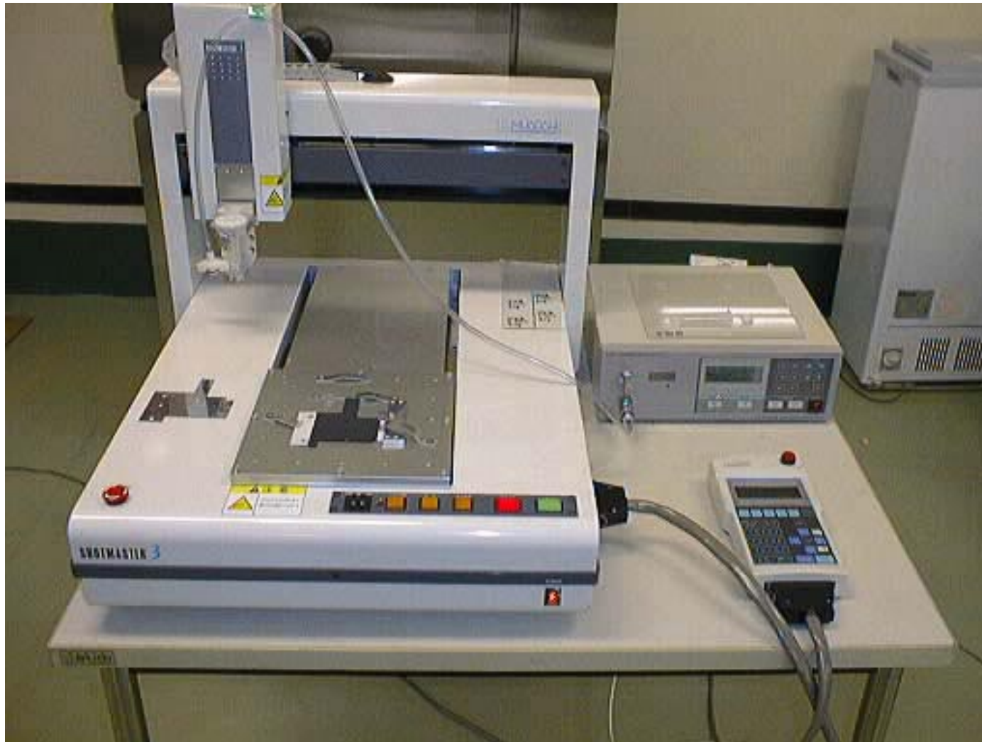
Figure 12: Glue dispensing system which is made of (1) a xyz stage where the baseboard is on the xy stage and a glue-syringe is attached on the z-axis, and (2) a dispensing controller.
