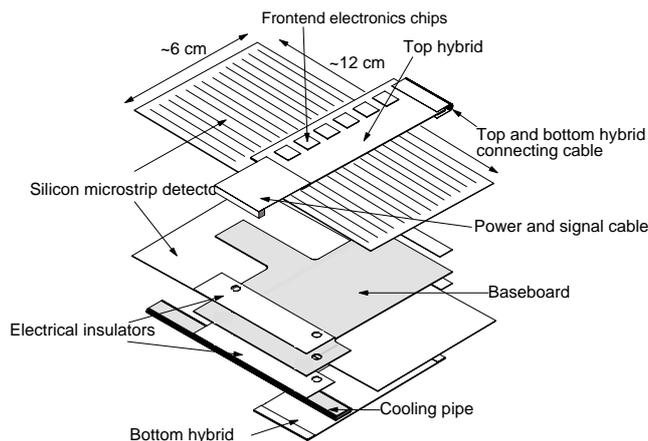
Figure 1: An expanded view of the Silicon microstrip detector module of the ATLAS SCT Barrel section.
