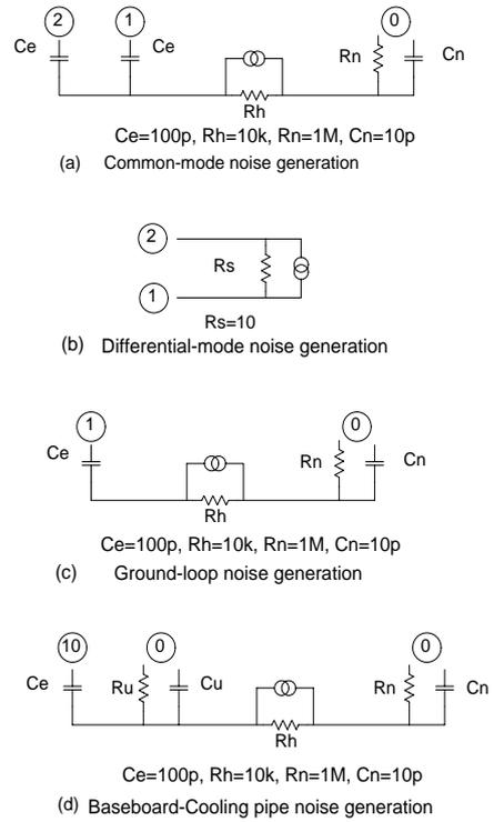
Figure 5: Implementation of pickup noise generation in the SPICE3 simulations: (a) Common-mode pickup on the bias power lines with the noise between the power supply leads, Nodes 1 and 2, and the amplifier ground, Node 0, (b) Differential-mode pickup in the bias lines, between Nodes 1 and 2, (c) Pickup on the ground-side bias line, between Node 1 and 0, and (d) Pickup on the cooling pipe, between the detector backside, Node 10, and Node 0, with an extra coupling to the Node 0 through Ru and Cu.
