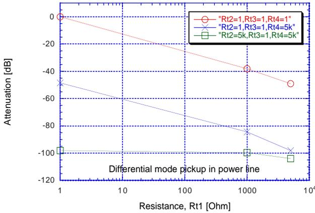
Figure 7: Attenuation of the differential-mode pickup noise in the bias power lines. The shunt capacitance,  $C_{t1}$ , was 20 nF.
