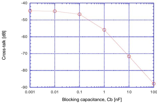
Figure 4: Attenuation of the crosstalk as a function of the blocking capacitance, Cb1 and Cb2
