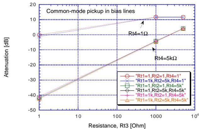
Figure 6: Attenuation of the common-mode noise in the bias power supply lines as parameterized with the filtering circuitry elements. The upper cluster of lines are the circle and cross, and the lower cluster of lines, the square, rhombus, plus, and triangle.
