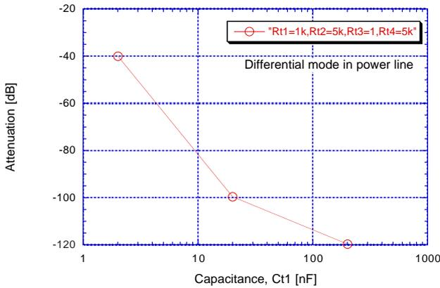
Figure 8: Attenuation of the differential-mode pickup noise in the power supply lines as a function of the shunt capacitance,  $C_{t1}$ .
