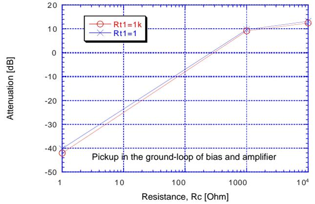
Figure 9: Attenuation of the pickup noise in the ground-loop of the bias line and the amplifier as a function of the shunt resistance,  $R_c$ .
