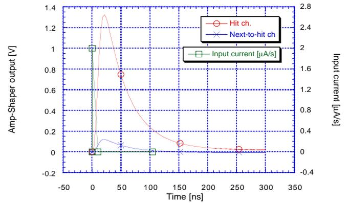
Figure 3: Response of the amplifier: Current in a strip (square), Amplifier output of the strip (circle), and Crosstalk output in the adjacent amplifier (cross)
