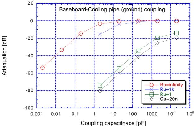
Figure 10: Attenuation of the noise in the cooling pipe as a function of the coupling capacitance between the cooling pipe and the baseboard, parameterized with the shunt resistance,  $R_u$ , or the shunt capacitance,  $C_u$ .
