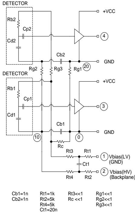
Figure 2: Simplified schematics of the detector-electronics chain modelled in the SPICE3 simulation. The nominal values of the components are also listed in the figure.
