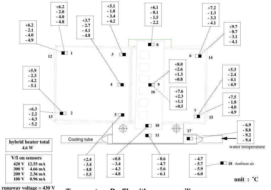
**Temperature Profile with power on silicon sensors**
