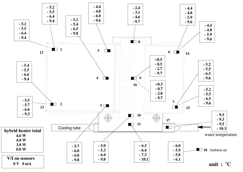
**Temperature Profile with no voltage on silicon sensors**
