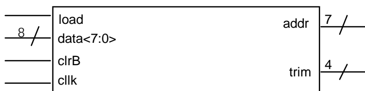
Figure 3.12A. Trim DAC Register Inputs/Outputs.
