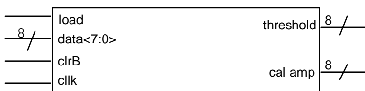
Figure 3.11. Threshold/Calibration DAC Register Inputs/Outputs.
