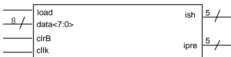
Figure 3.12. Bias DAC Register Inputs/Outputs.
