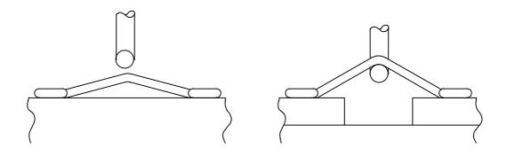
FIGURE 2011-3. Flat loop wire pull testing.
