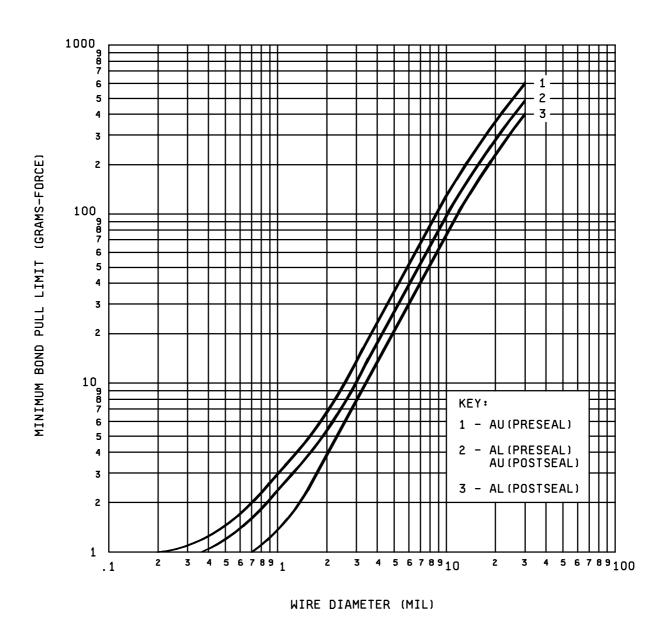
NOTE: The minimum bond strength should be taken from table I. Figure 2011-1 may be used for wire diameters not specified in table I.
